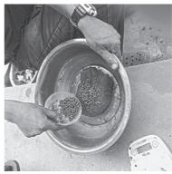
The pulverized brick was mixed in to the pathaipet, adjusting water amounts as explained above. The resulting mixture of pathaipet and brick was used to
